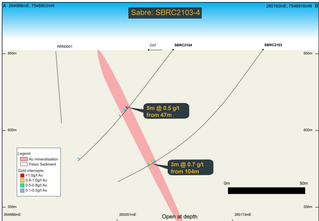
Figure 3 – Sabre drilling section highlighting significant results from SBRC2103 and SBRC2104 at Reynolds Range.
