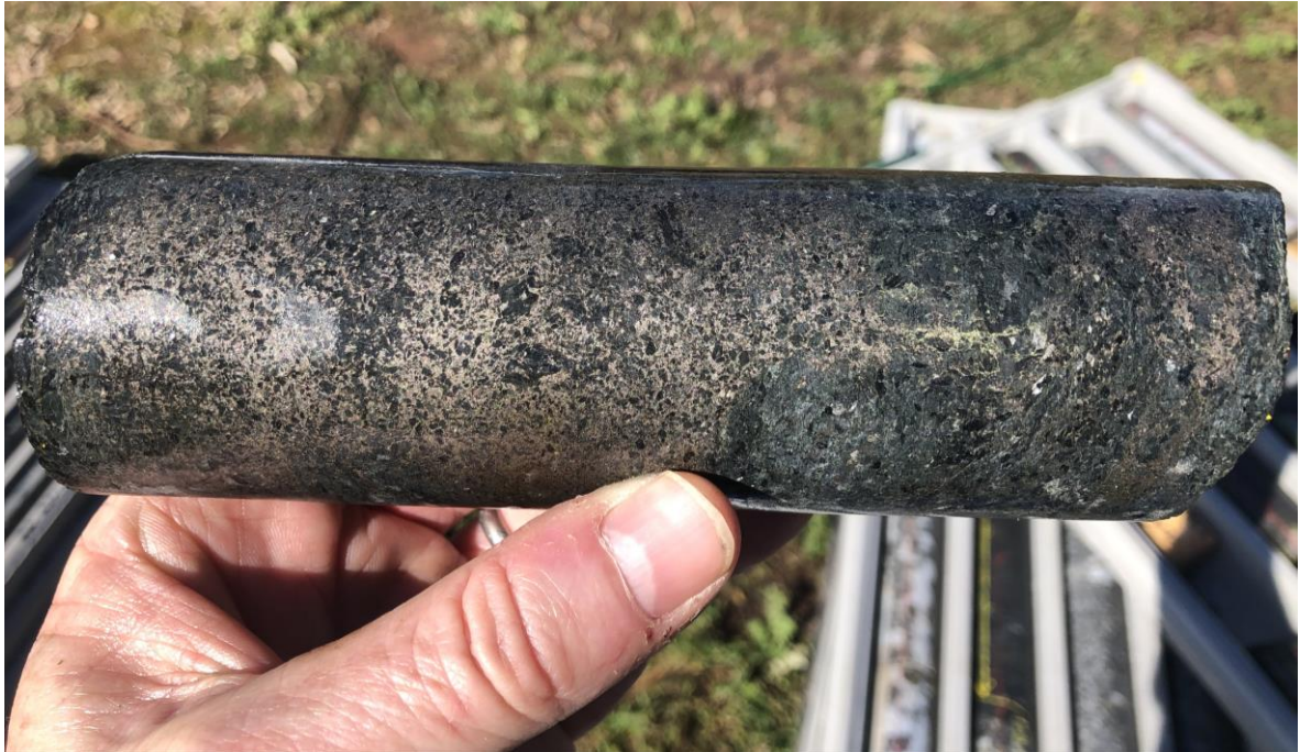
Figure 1 - Semi-massive sulphides in ultramafic – pyrrhotite and minor chalcopyrite at 141.3m in MNEWDD002
