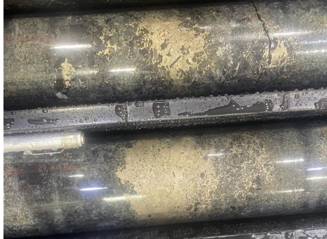
Semi massive 3 phase sulphides in cumulate gabbronorite, 576.8m
