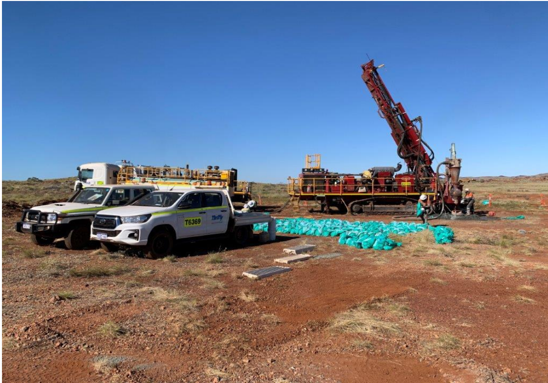
Figure 7: Current drill programme - Schramm track mounted rig drilling hole ARC319
