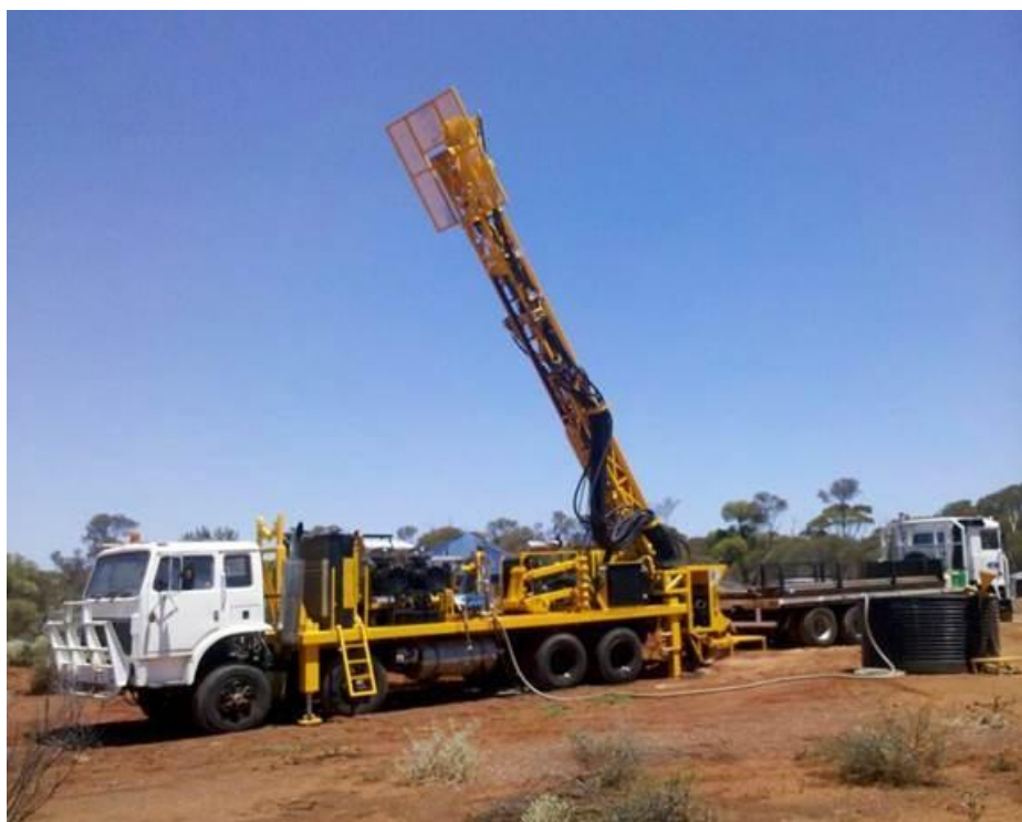
Figure 1: CEO, Andrew Pumphrey, owned multi-purpose RC and diamond drill rig
