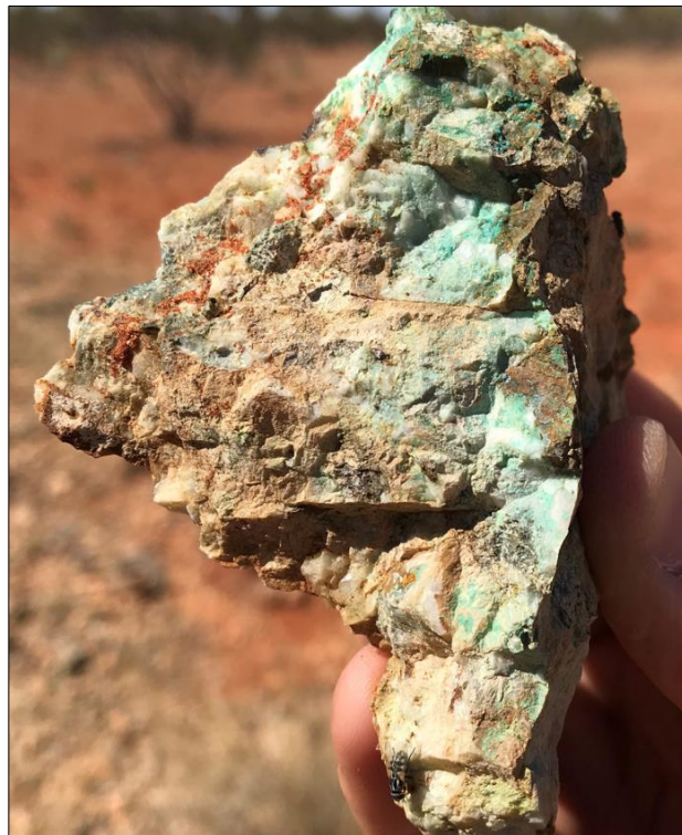
Figure 9: Photo of rock sample JE0097 before it was submitted for assaying. It was sampled because of its visible copper mineralisation but was found to contain high levels of gold and bismuth as well, 3.21g/t gold, 1.89% copper and 0.28% bismuth.
