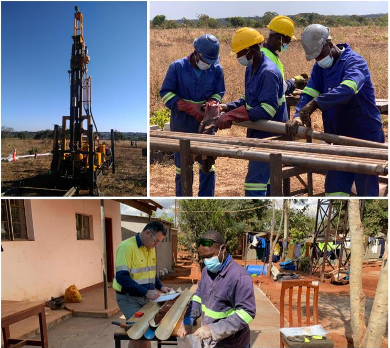
Figures 1, 2 & 3: Core rig in action at Kasiya (top left). Drill team extracting the core from the drill rods (top right). Sovereign's Managing Director, Julian Stephens in Malawi inspecting the core.
