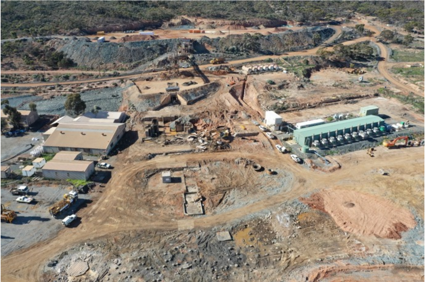
Photograph of the Phoenix plant site with the processing plant, gold room, and other redundant building infrastructure removed.
