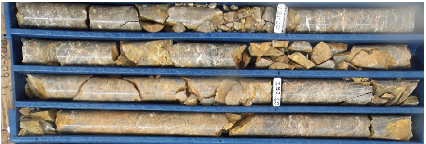
Figure 12: RP01 core tray photo ( \pm 280.6\text{m} - 283.9\text{m} ) of highly brecciated and oxidised Jumasha Formation limestone.
