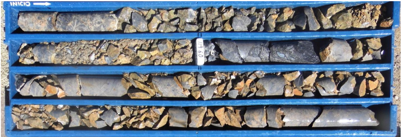
Figure 13: RP01 core tray photo ( \pm 118.1\text{m} - 123.1\text{m} ) of high fractured silicified Jumasha Formation limestone with calcite-Mn oxide veinlets and trace amounts of pyrite.
