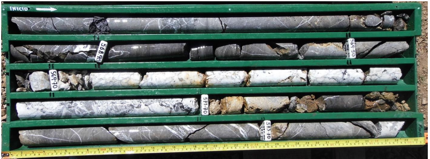
Figure 9: RP01 core tray photo (±567.70m-574.0m) of highly altered Jumasha Formation effected by quartz and calcite veins and veinlets.
