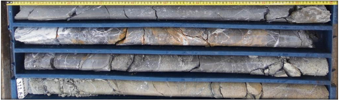
Figure 11: RP01 core tray photo ( \pm 319.8\text{m} - 323.1\text{m} ) of highly altered and brecciated/veined porphyritic diorite dyke.
