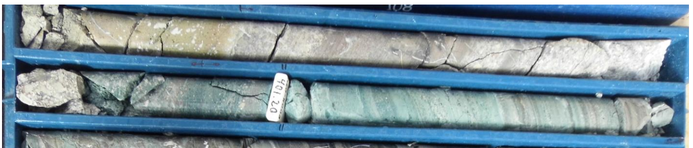
Figure 10: RP01 core tray photo (±399.8m-401.9m) of a highly altered andesitic sill effected by quartz and pyrite veins and veinlets.
