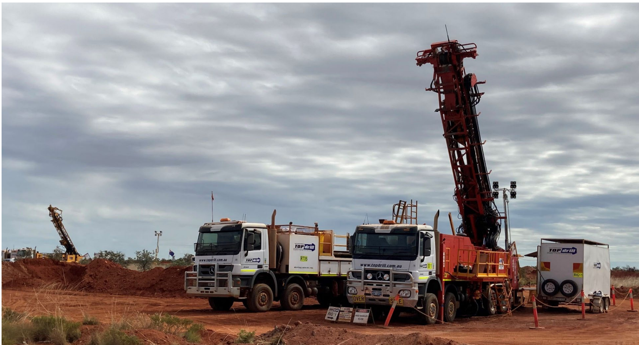
Figure 2 TopDrill diamond rig drilling HERC889D, targeting approximately 160m below HERC851D on Section 28720E. Second diamond rig (LHS) is drilling on section 28660E aiming to extend the zone 80m to the west
