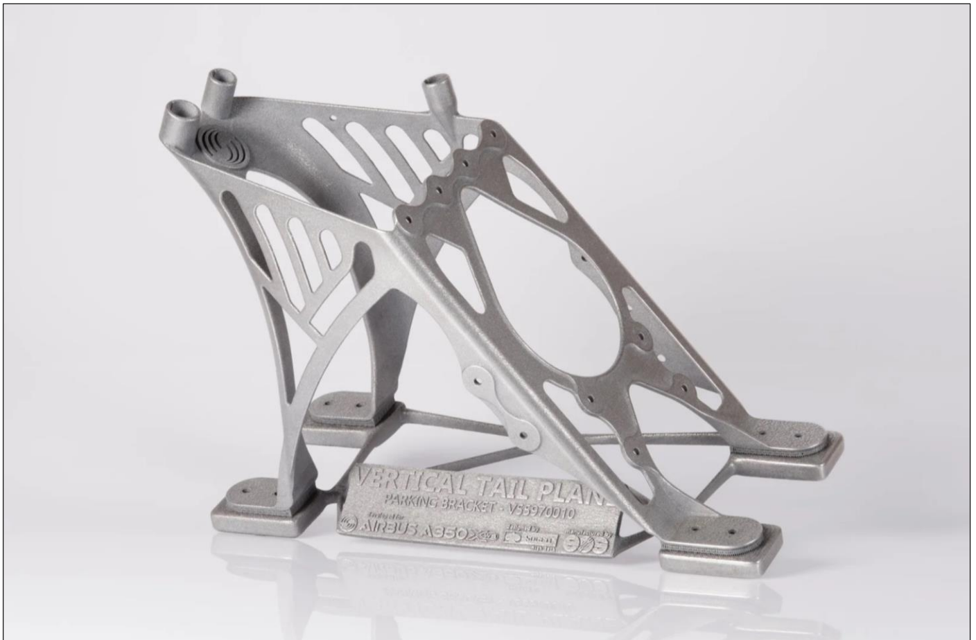
A350 titanium cable mount on the front spar of the vertical stabilizer made with EOS 3D printer.
