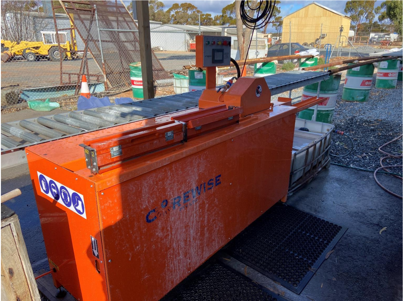
Image 4 – Recently delivered core-cutting saw installed at our Kambalda yard.
