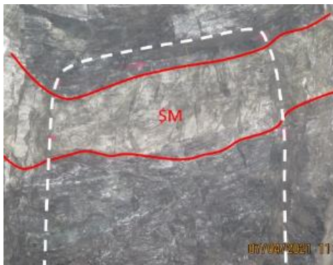
SBA 788 south ore drive (3.5mW x 3.5mH) with a face grade 3.6% Ni
