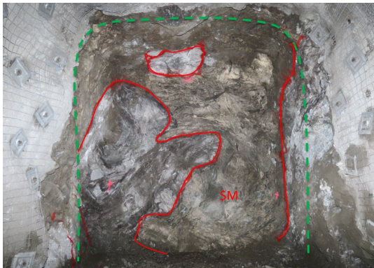
110 south ore drive (4.0mW x 4.5mH) with a face grade 4.6% Ni
