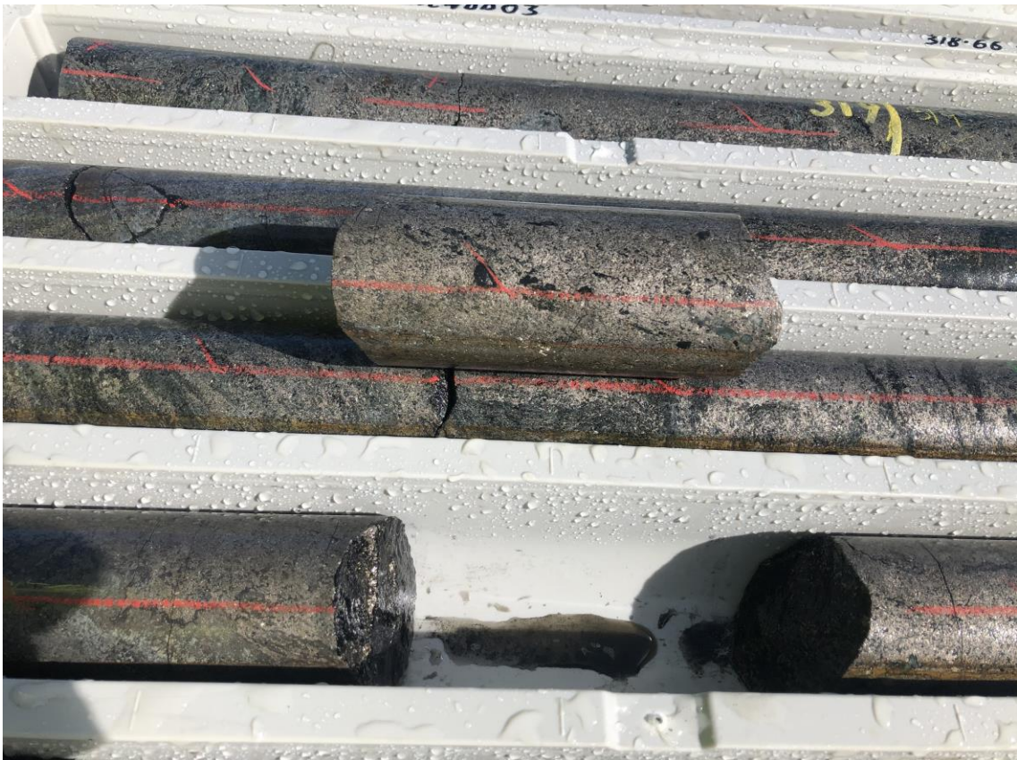
Figure 1 – Massive sulphides – pyrrhotite and minor chalcopyrite at 321.5m in MNEWDD003
