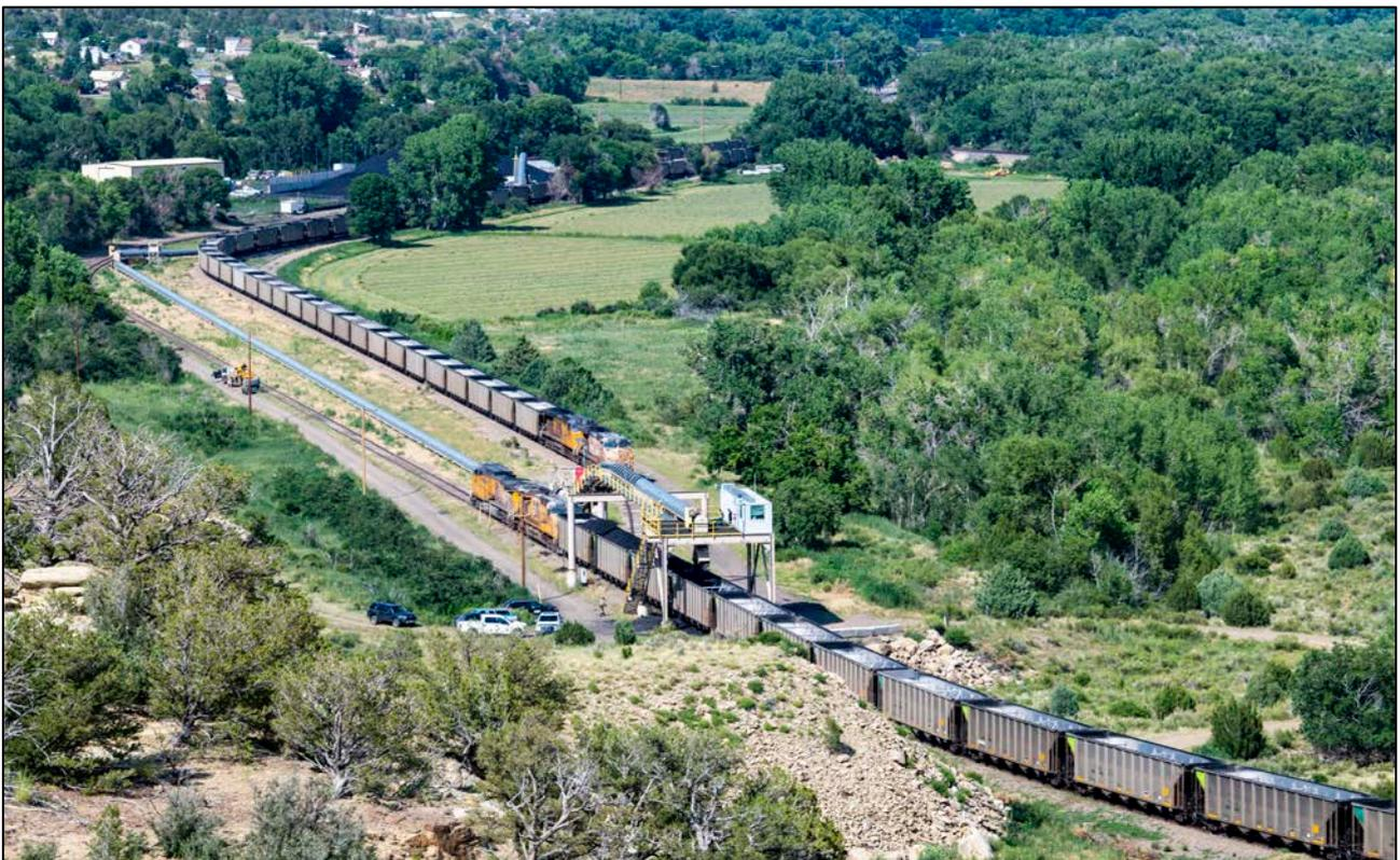
Image: New Elk coal loading with the train split in half each with two locos due to the length of the siding
