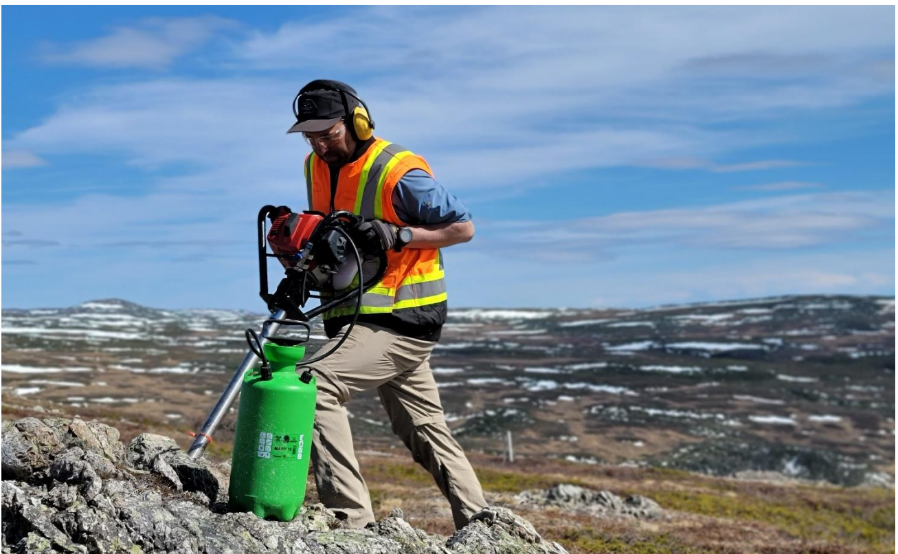
Figure 1: Hand-held power-auger drilling sampling outcrop
