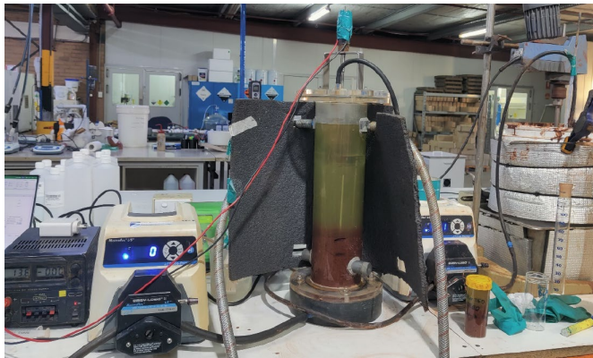
Dynamic Leach Discharge Thickening
