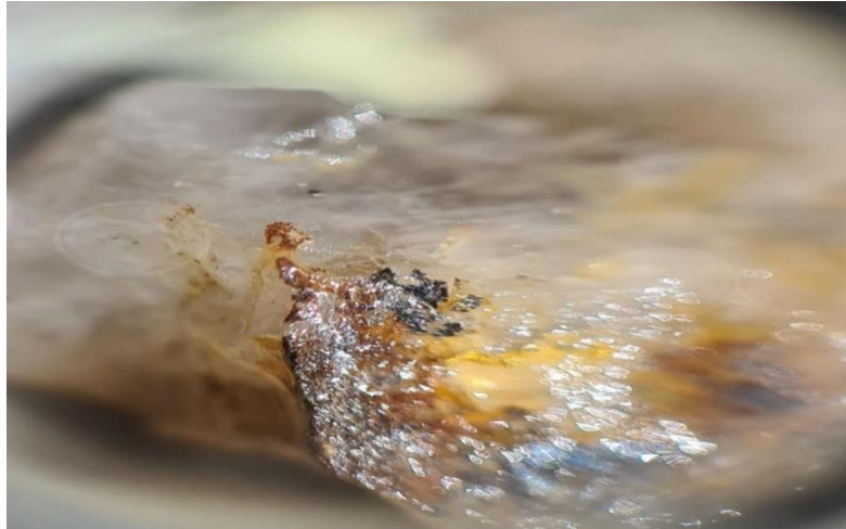
Figure 1: Free coarse gold hosted within quartz vein (yellow colour) assayed 10.93 g/t Au
