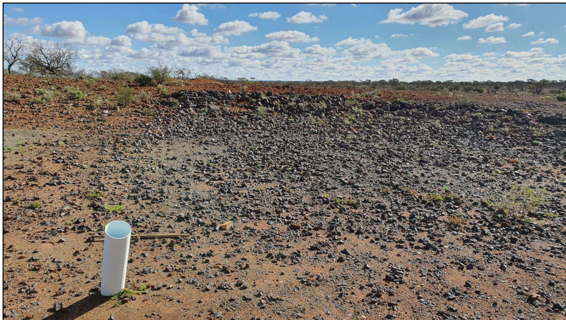
Figure 10. Photograph of Gossan 1 (dark rock), showing a historical drillhole designed to test beneath it.
