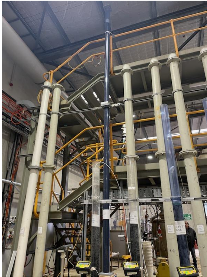
Figure 4 - 5.5 metre column (in the centre of the image)
