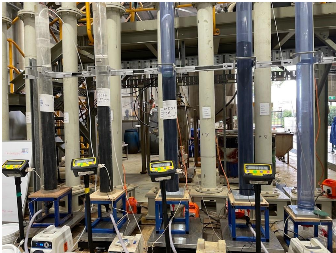
Figure 2 - Counter-current 1m leach column arrangement showing four columns filled and leaching and one empty column to be filled
