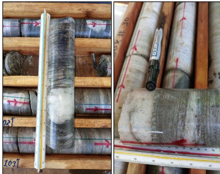
Figure 8 –Drill core from BBDD001 showing intervals of highly altered host rocks and quartz veining, both with significant visible sulphide mineralisation (pyrite, chalcopyrite, pyrrhotite). Left: ca. 101m Right: ca. 106m
