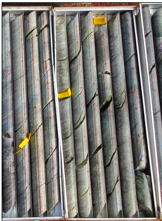
Figure 4: Strongly Sheared Granodiorite (Altered to Quartz Feldspar Sericite Schist) with Quartz Veins and Veinlets (c. 5%) 5 -10% Pyrite, 1-2% Chalcopyrite and 5-10% pyrrhotite mineralisation from hole CKDD010
