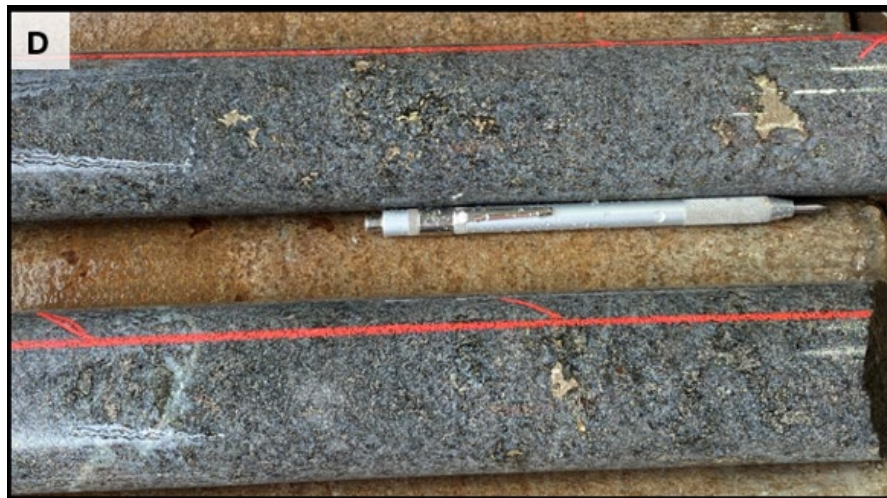
Coarse three-phase Po-Cp-Pn blebs and carbonate veinlets in gabbro-norite at 464m in 21AFDD104.
