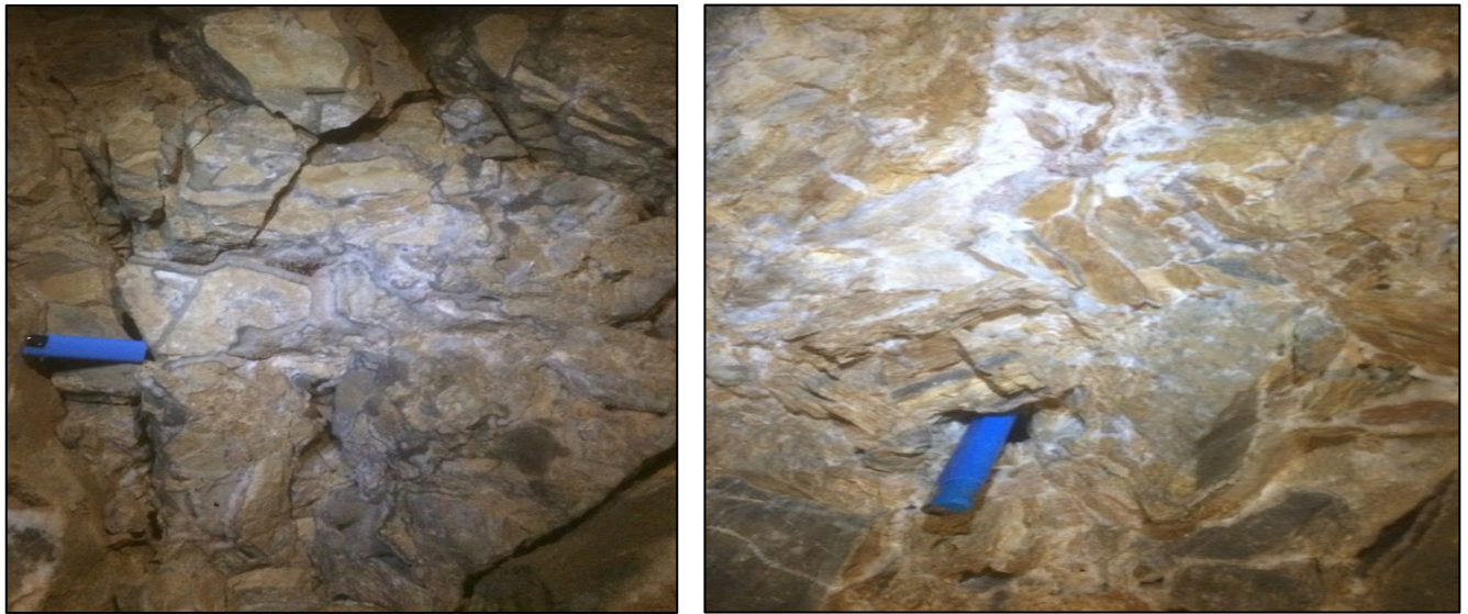
Figure 2 - Breccia ore: Open space & drusy quartz, layered & minor sulfides matrix, carbonate clasts (left) & Silica flooded matrix minor sulphides with carbonate clasts (right)
