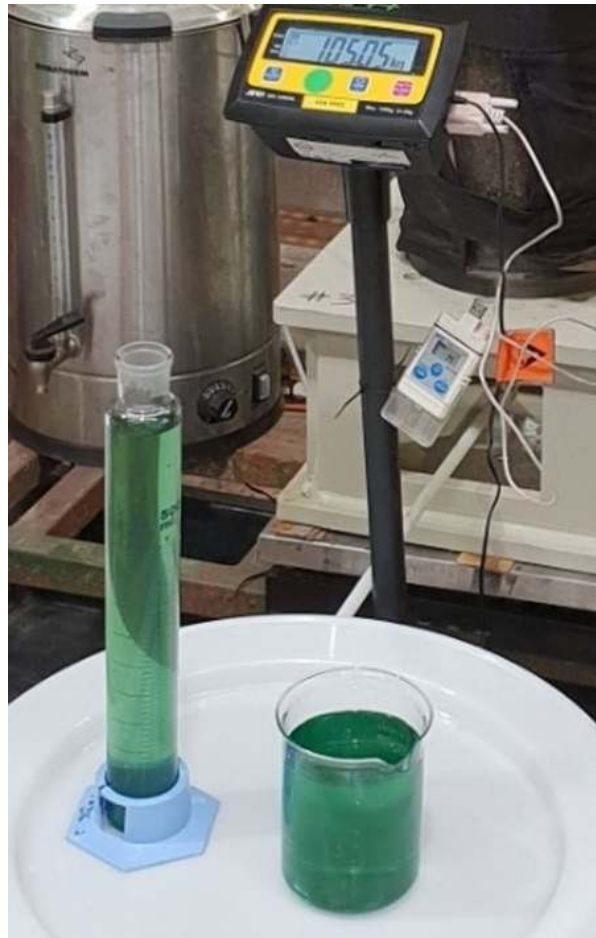
Image 5 | Copper sulphate solution from Nifty test-work column 1
