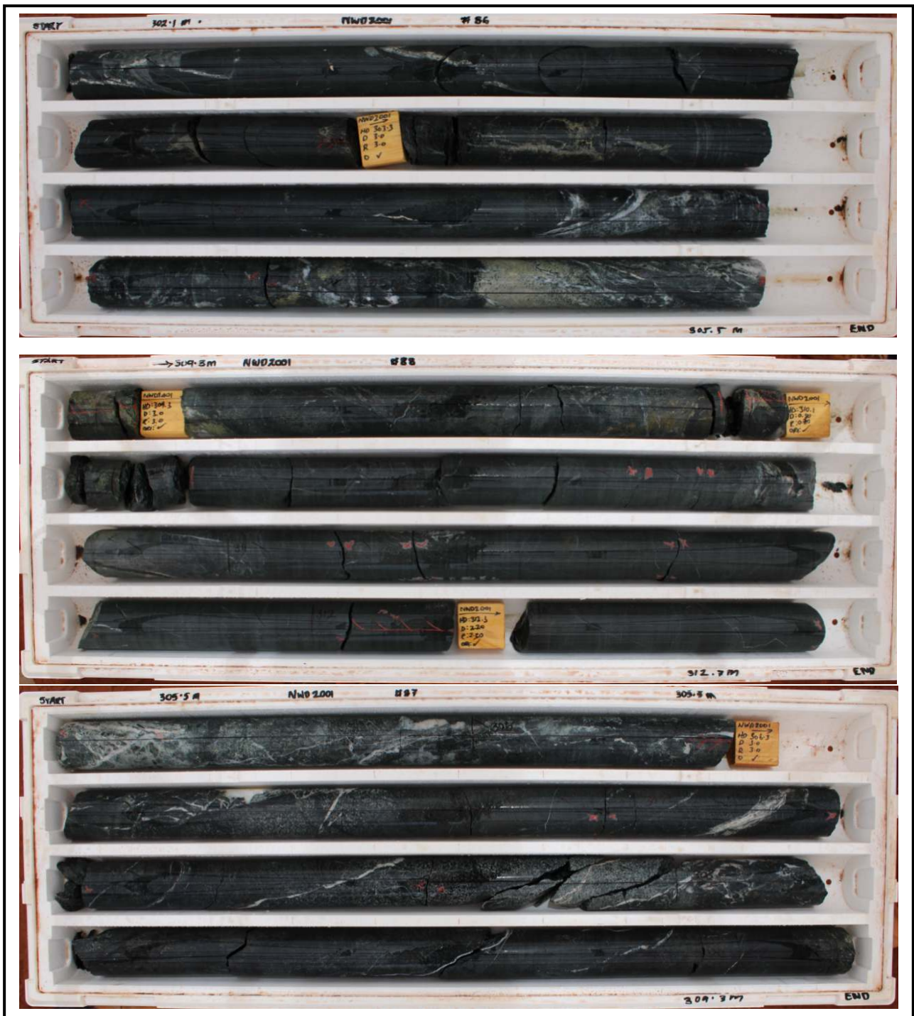
Image 7 | NWD2001: 303.0m to 312.0m; 9.0m @ 392 Ag g/t crackle breccia silver sulphide mineralisation, including 2.0m @ 1,470 Ag g/t from 306.0m.
