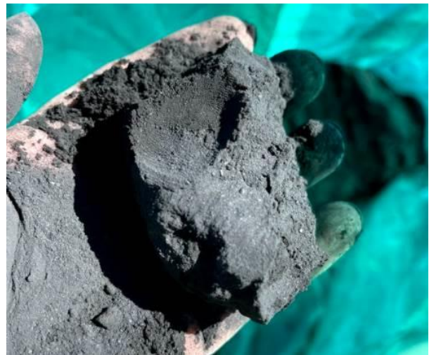
Figure 6a (left): Rich Chalcopyrite Mineralisation (88-89m, 5.8% Cu – WCRC021); and Figure 6b (right) Rich Chalcocite Mineralisation WCRC006 (18-19m) at Powder Hill, Grading 9.5% Cu.
