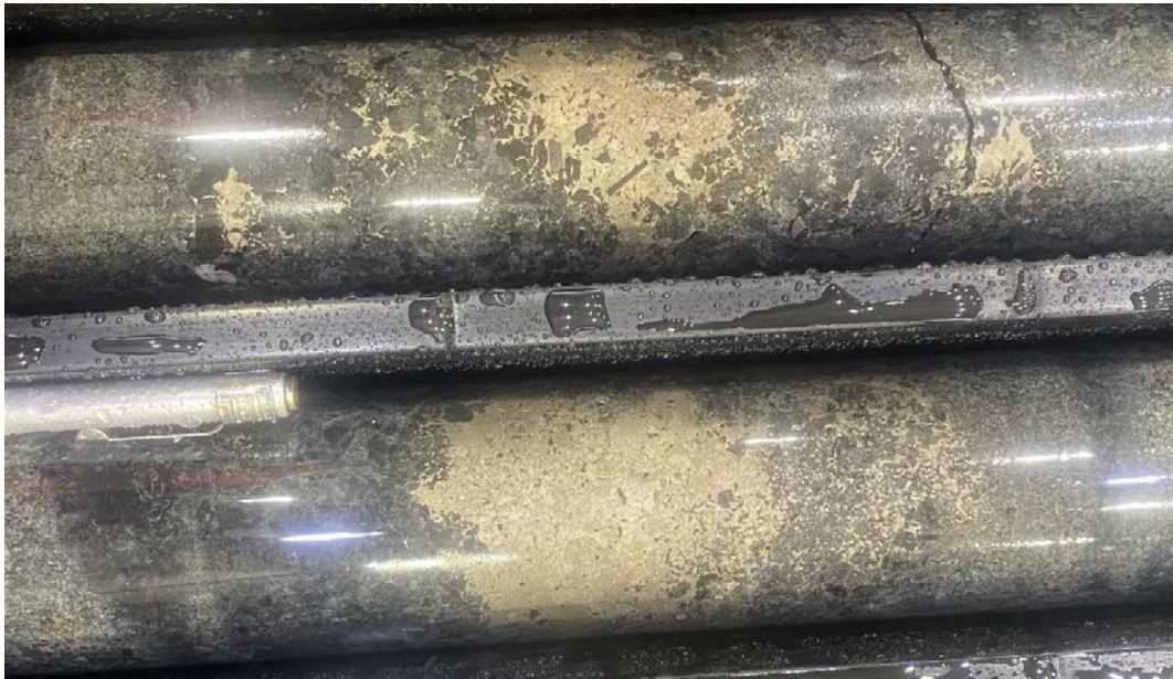
Figure 28: Semi massive 3 phase sulphides in cumulate gabbro, 576.8m
