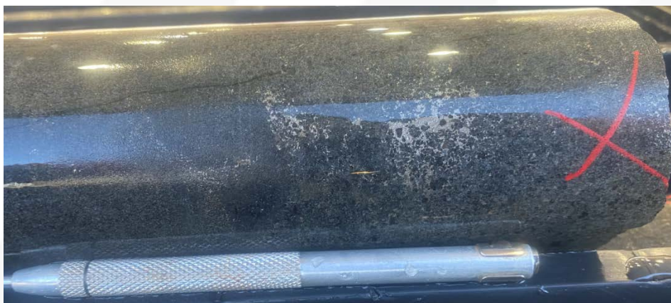
Figure 26: Disseminated pyrrhotite in mesocumulate gabbro norite, 222.5m
