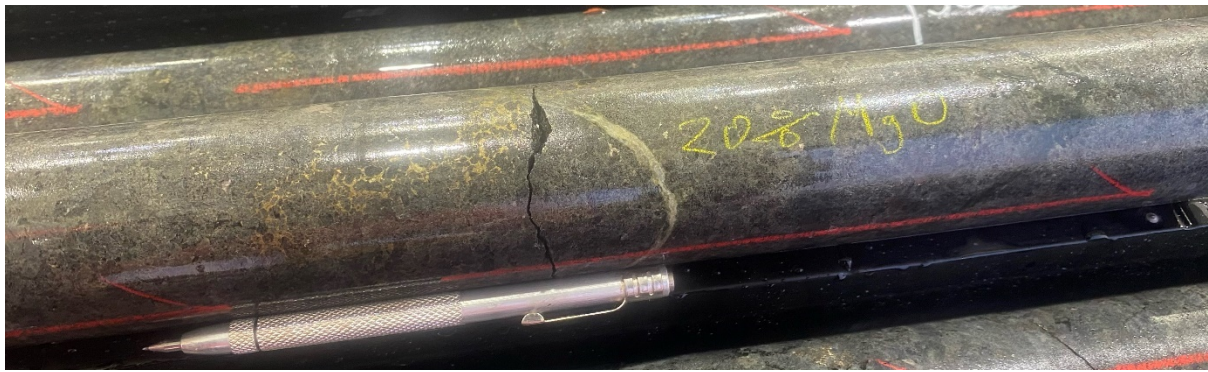
Figure 24: Mesocumulate websterite with disseminated 2 phase sulphides (Po>Cp), 503m
