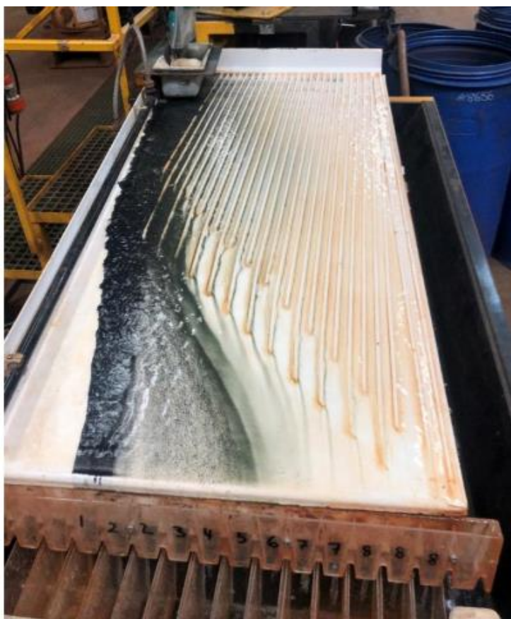
Figure 2: Gravity Separation Table – Dark, heavy material concentrated to left containing titanium feed
