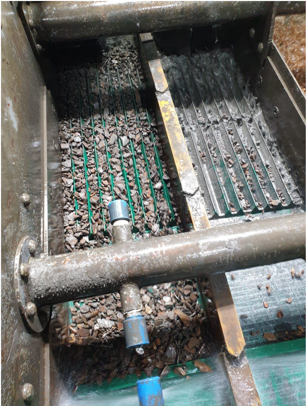
Figure 4: Sample MIN06039 (DID) DMS Test work @ SG 3.0 Lumps (product screen on left, discard screen on right)
