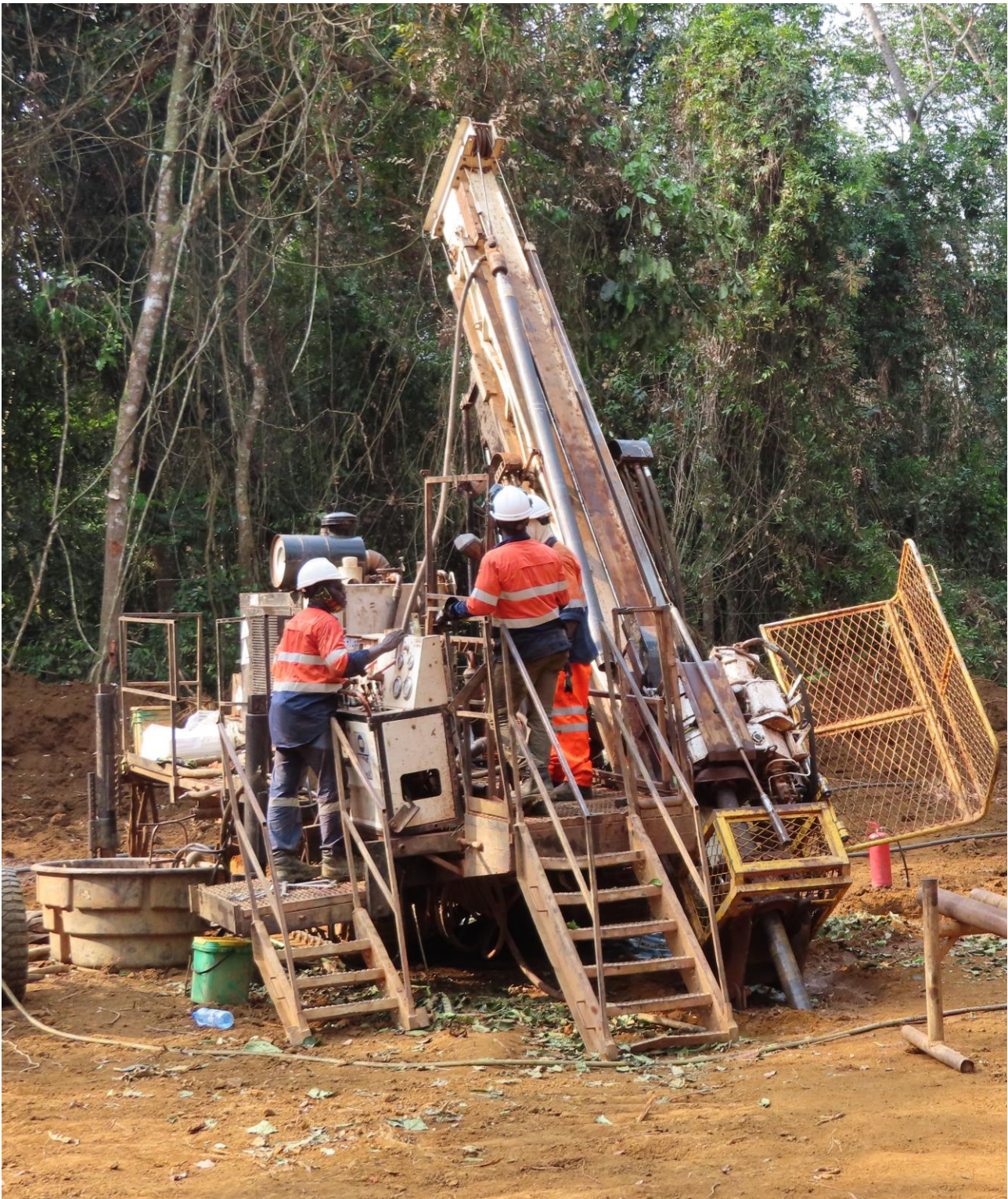
Figure 5: Boart Longyear LF 90 diamond drill at Bandjougoy prospect on 30 June 2021 (Drill Hole BWDDH0013)
