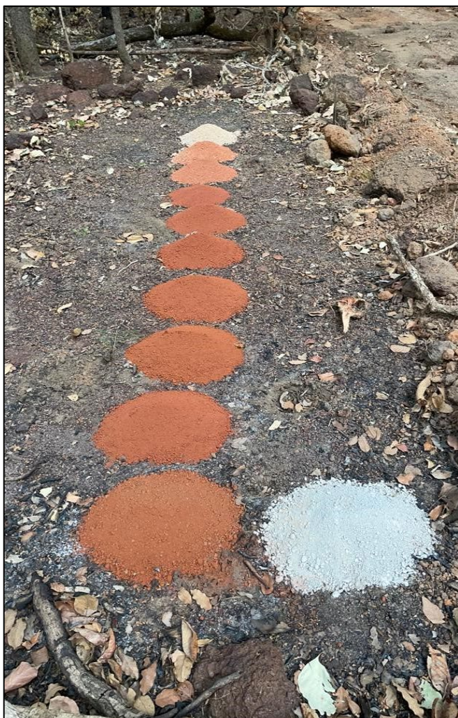
Figure 3. Typical lateritic weathering profile encountered in the auger holes at Kada. Bottom of hole samples for gold analysis collected in saprolite beneath the lateritic horizon.
