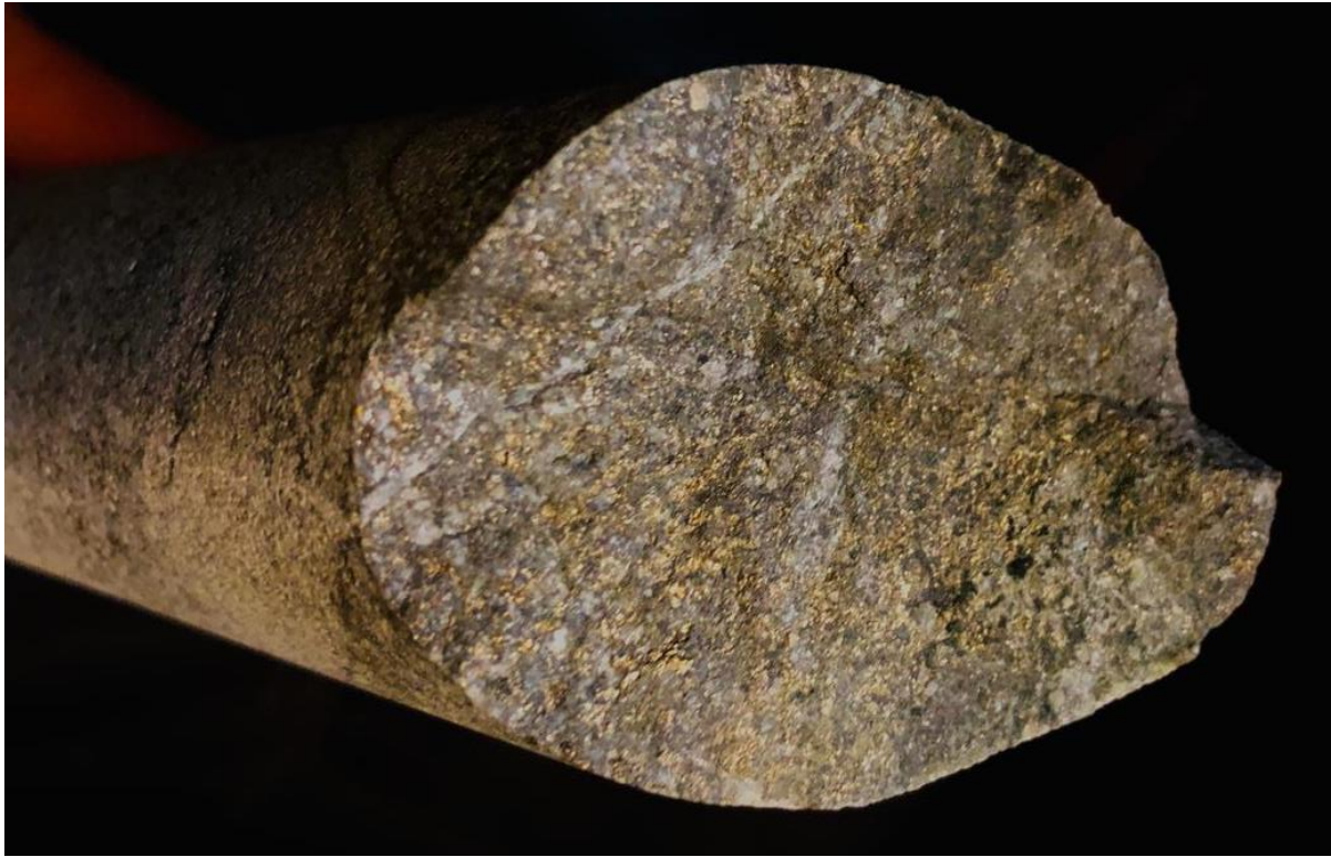
Figure 1 Sulphide mineralisation in drill-hole MIDD003 at 97.43m drilled depth.
