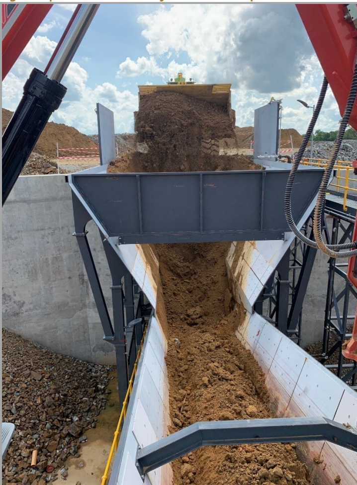
Figure 6 | Crushed ore conveyed to the stockpile
