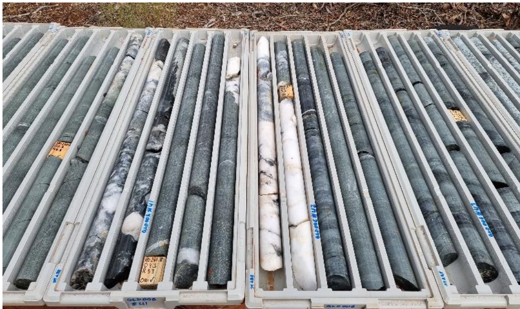
Figure 1: QLD006 Quartz biotite-tourmaline veining with pyrrhotite and chalcopyrite
