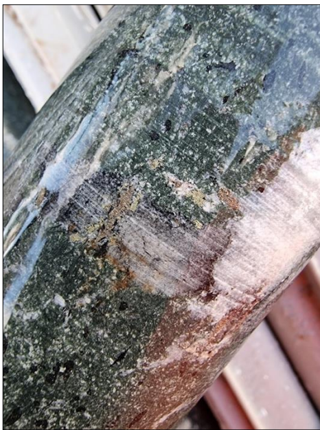
Figure 3: QLD008 Quartz Tourmaline Sulphide vein in an altered mafic close up
