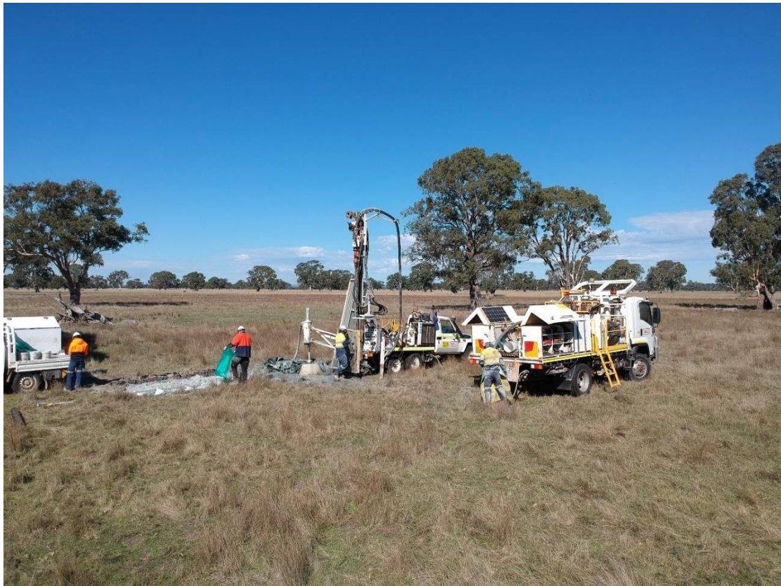
Photo 5. Air-core drilling at the Toora West prospect.
