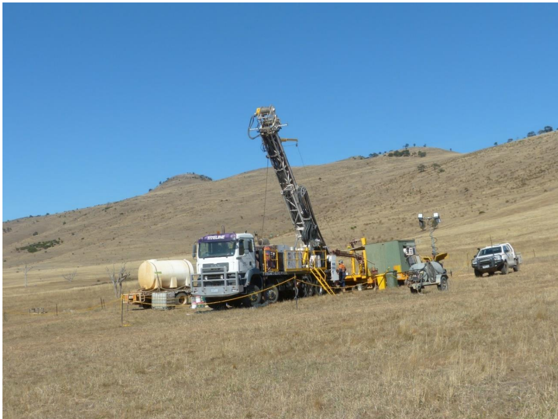
Photo 6. Diamond Drill Rig at Mount Ararat.
