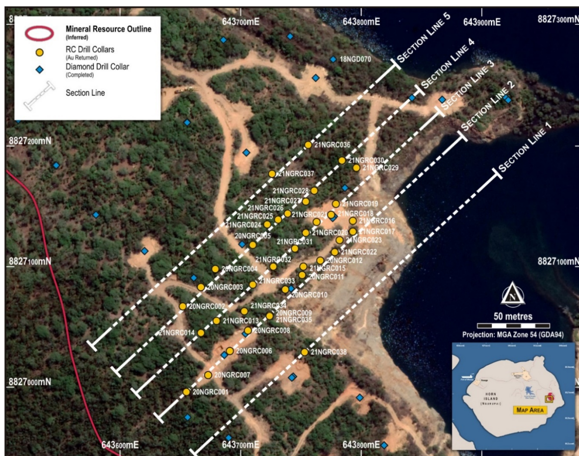
Figure 1 AQX Phase 1 RC, interim Phase 2 (x 3 holes) and diamond drill hole collar locations adjacent to the historic 1980s gold mine open cut pit area.
