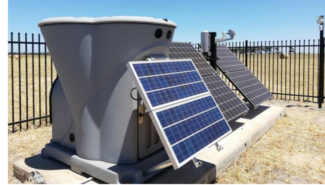
SODAR solar unit installed for 2022 pre-feasibility study into the establishment of a Renewables Energy Hub
