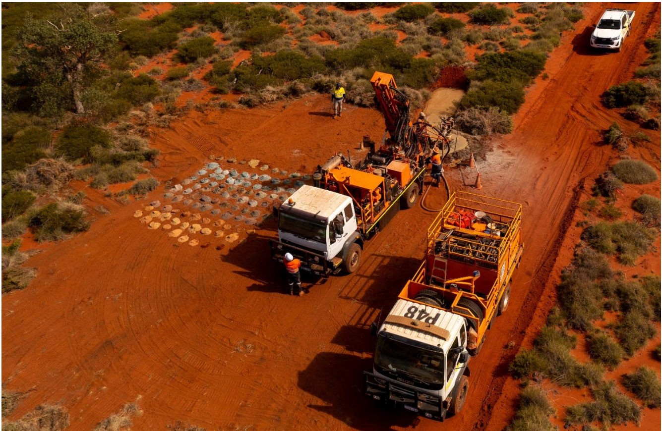
Figure 1: Air-core drilling at Roberts Hill
