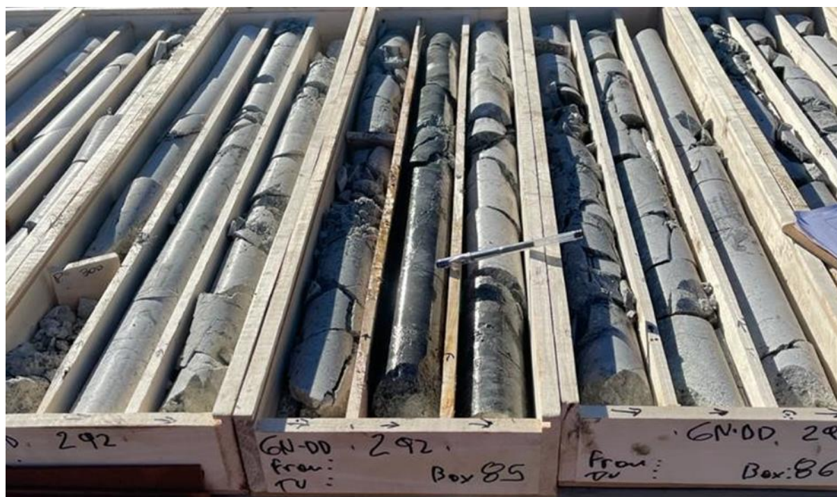
Photo 3 : GNDD-292 sulphide interval 233 metres downhole (skarn alteration 15% pyrite 5% sphalerite)
