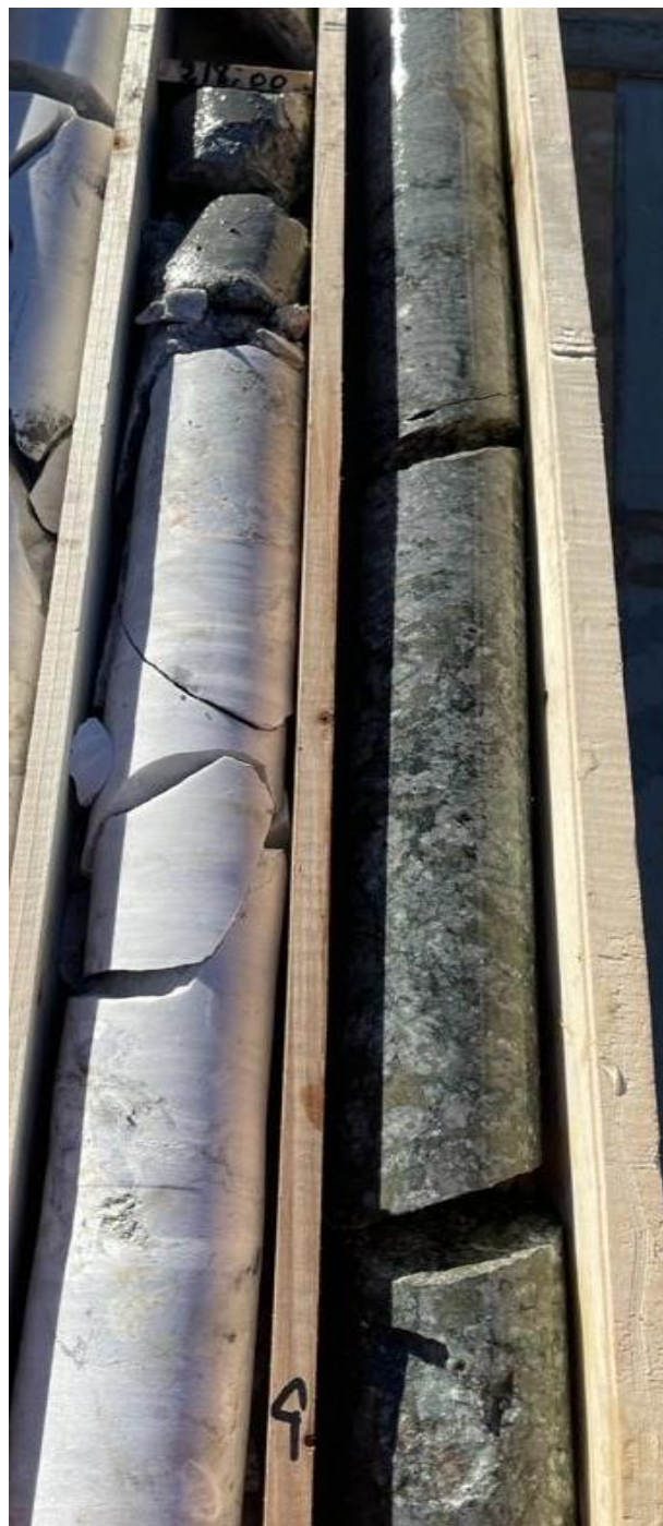
GNDD-292 - sulphide Interval 218-219m
