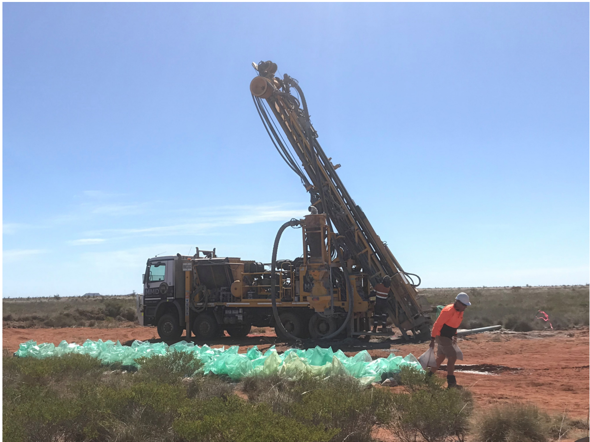
Figure 1. Photo of the RC drill rig at the Bastion Prospect, Strelley.
