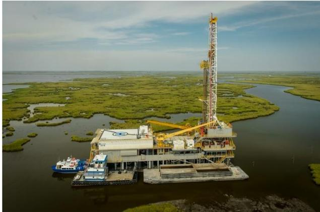
*Shallow-draft barge drilling rig*
