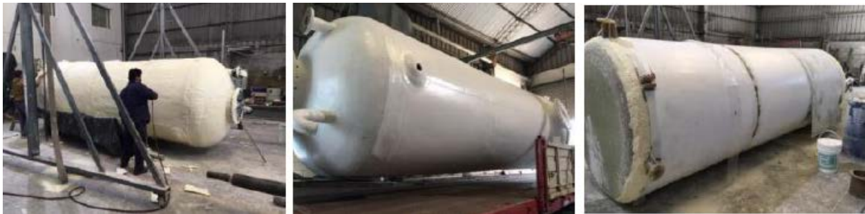
Figure 3. Rincon Lithium Project – 2,000tpa Operation Fabrication Works (Process Tanks & Reactors)
