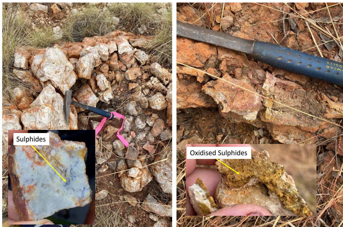
Figure 3 Left: Quartz Adularia veining with sulphides at Tunganary; Right: Quartz breccia and veining with oxidised sulphides at Middle Branch.
