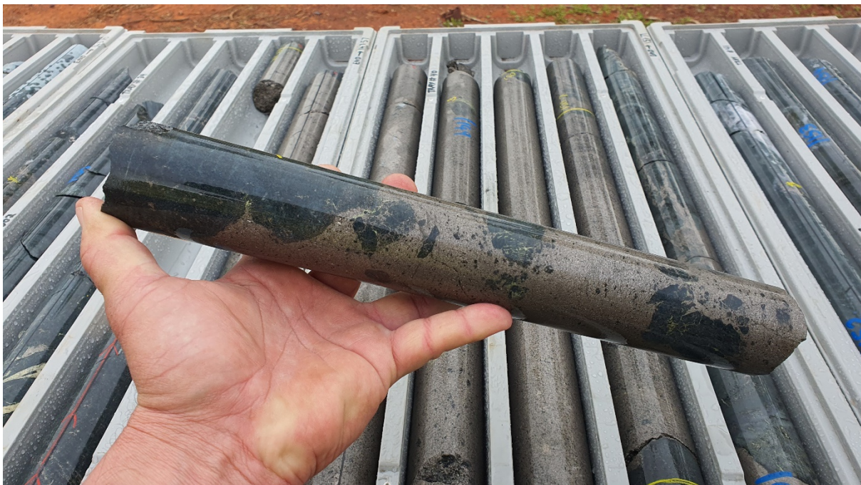
Figure 1. Photograph of semi-massive sulphide from the hangingwall contact of the massive sulphide starting at 146.4m downhole. This illustrates the interaction of a sulphide melt with the country-rock (in this case ultramafic). The rest of the massive sulphide zone can be seen in the background.
