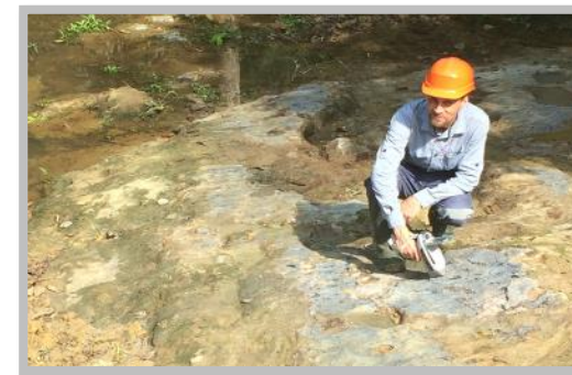
Outcrop of mineralised sandstone at the Dikaki embayment containing approximately 20 – 40 % galena and sphalerite
