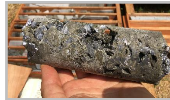
Mineralisation in hole DKDD013 at Dikaki (2018) – showing coarse textured galena, sphalerite and marcasite within the basal carbonates unit
