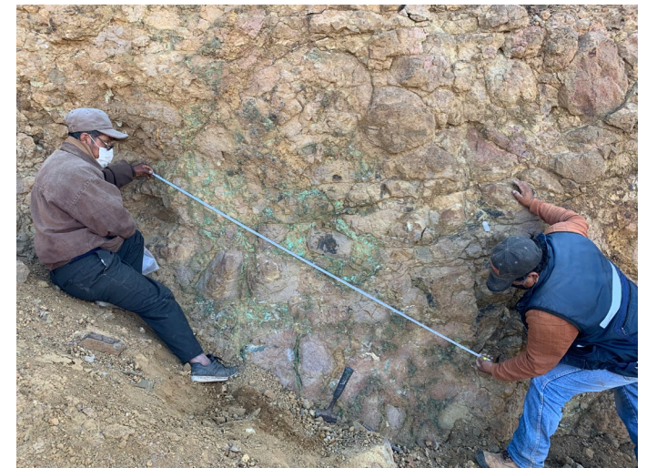
Cobremani: measuring sample area. Sample 33: 65.6 g/t Ag and 4.97% Cu- Channel
