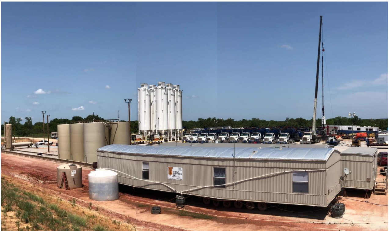
Figure 1. Completion equipment on site with hydraulic stimulation having now commenced
