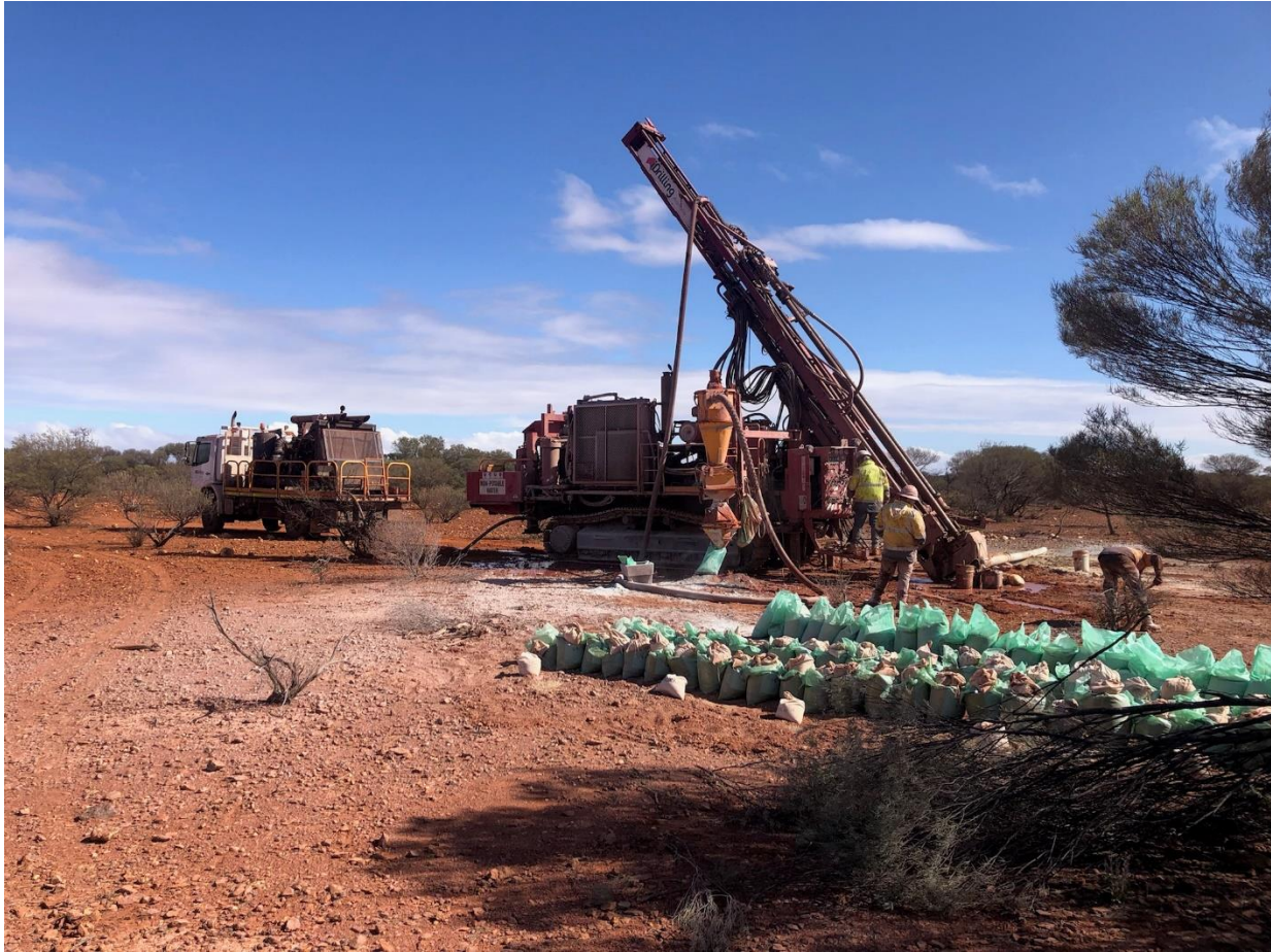
Figure 1: RC Drill Rig on site at Pharos
