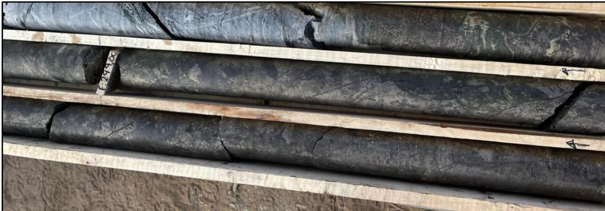
Photo 1 - Footwall Zone mineralisation from 297-300 metres in GNDD-314 (assays pending)
