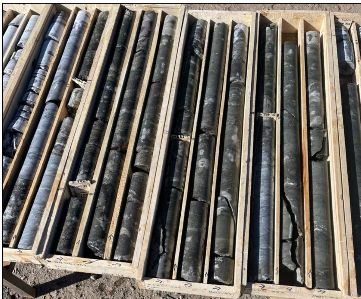
Photo 4 - Intersection of the Sentazon Manto from 142-155 metres downhole in GNDD-352 (assays pending)
