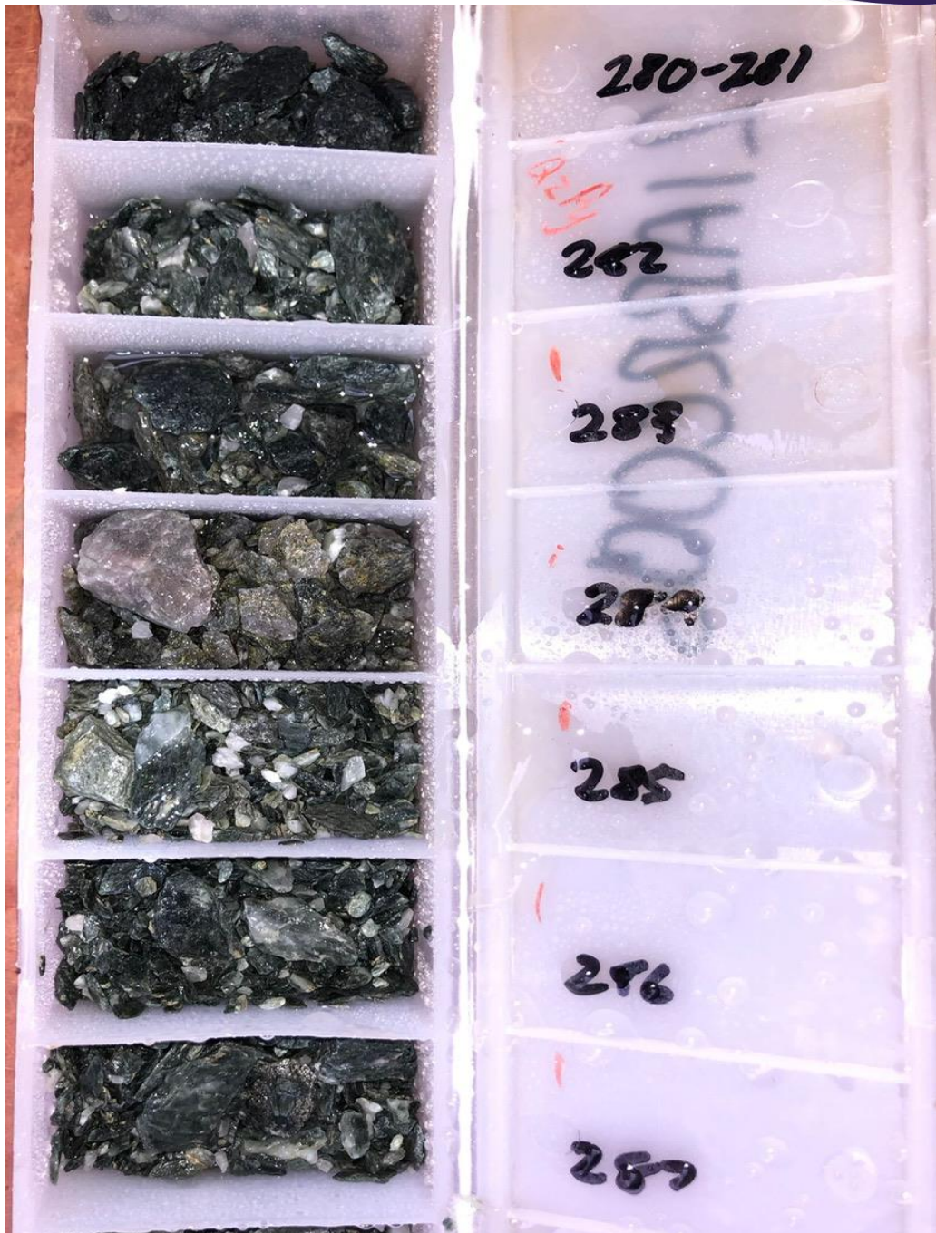
Figure 2 – Representative Sample Chips of Mineralised Alteration Zone (21ABRC006 280m to 287m downhole).
