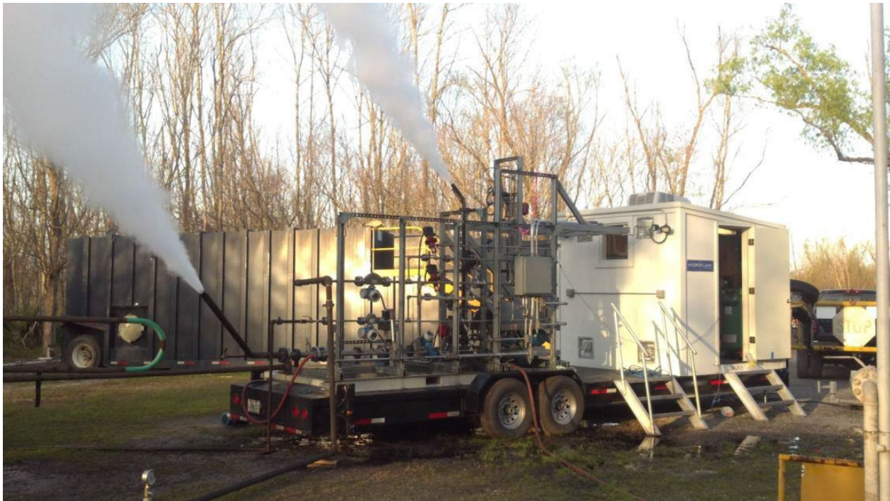
AVS' Superheated Steam Generator
