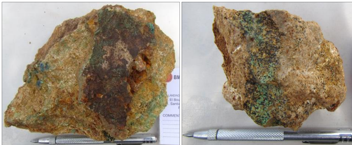
Figure 8: Sample specimen photos of BM-01032 (left) and BM-01033 (right). At Cachillusca the mineralisation occurs in structures with manganese oxides and quartz veinlets. Coordinates listed in Table 2 and approximate locations shown on Figure 9.
