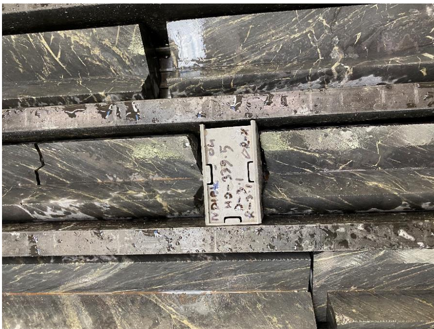
Figure 12: Photo of core from Government drill-hole NDIBK04, core depth is 339.5m. The core has been cut in half and one half has been cut again. A quarter-core sample every metre has been submitted for multi-element analysis. THE CORE IN THIS PICTURE IS FROM GOVERNMENT DRILL HOLE NDIBK04 - IT IS NOT THE PROPERTY OF THE COMPANY - PENDING ASSAYS BEING CONDUCTED BY THE GOVERNMENT WILL BE PROVIDED TO THE PUBLIC VIA GOVERNMENT AGENCY WEBSITES.
