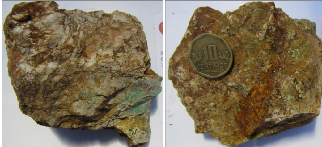
Figure 7: Secondary Cu mineralisation (malachite and chrysocolla) from Ajo Orjo. At Ajo Orjo the mineralisation occurs in brecciated volcanics with quartz and calcite veinlets. The assay results of these samples are not currently available.
