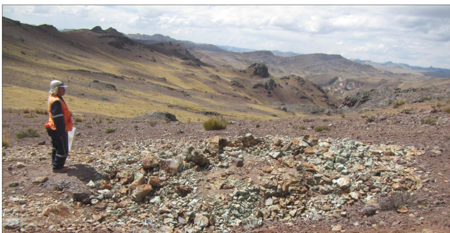
Figure 4: Outcrop photo showing extensive secondary copper mineralisation at Cerro Vicuña. Samples BM-00962 (a 3m x 5m composite sample) and BM-00963 (a 2m x 1m composite sample) were taken from this location. BM-00962 returned 4.55% Cu and 23g/t Ag. BM-00963 returned 3.73% Cu and 6.89g/t Ag.
