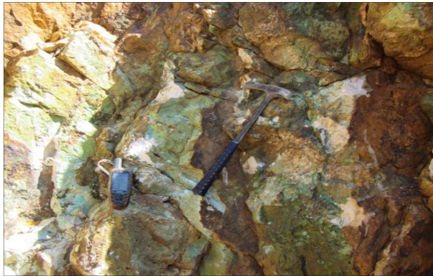
Figure 5: Outcrop photo showing brecciated structures hosting massive secondary copper mineralisation (malachite and chrysocolla) from the Enclave area of Riqueza (concession name Uchpanga III, previously reported in ASX announcement of 20 October 2020. Assay results from this outcrop include 4.54% Cu, 50g/t Ag (BM-00956) and 3.48% Cu, 82g/t Ag (BM-00957).
